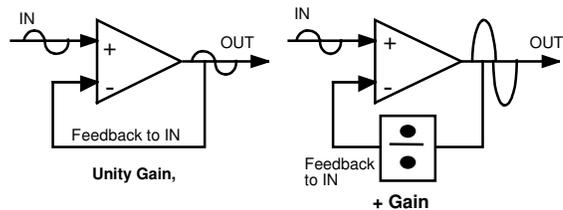
The job of the amplifier is to offer up as much current as it takes to create the right voltage drop in the load. The lower the load impedance, the greater the current to get the voltage, good old Ohms law in action. When the voltage drop in the load is equal to amplifier output then the current stabilizes. Prior to that, the amplifier will do whatever is necessary with the current to get the load's voltage right. The
